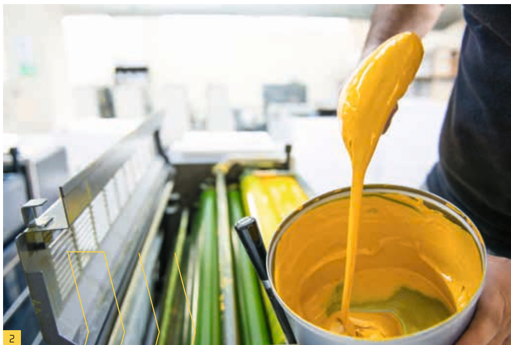
1+2 The LED UV colour series are matched to the wavelength ranges 385 and 395 nm as well as to H-UV applications.
